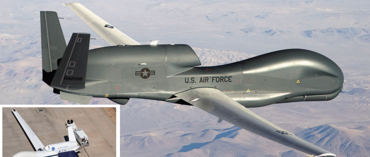
FIRST FLOWN IN 1998, THE U.S. AIR FORCE NORTHROP GRUMMAN RQ-4 GLOBAL HAWK IS STILL RELIED UPON AS A REMOTELY-CONTROLLED RECONNAISSANCE DRONE THAT IS SUITED FOR VERY HIGH ALTITUDE, LONG DURATION FLIGHTS. PILOTING THESE VEHICLES FROM THE GROUND HAS ALLEVIATED THE CONSTRAINTS OF HUMAN ENDURANCE WITHOUT THE RISK TO LIFE. GLOBAL HAWKS HAVE ALSO BEEN USED EXTENSIVELY BY NASA FOR HURRICANE AND SEVERE STORM STUDIES UNDER THE HS3 MISSION. IMAGE CREDITS: U.S. AIR FORCE/BOBBI ZAPKA/NASA GODDARD SPACEFLIGHT CENTER
