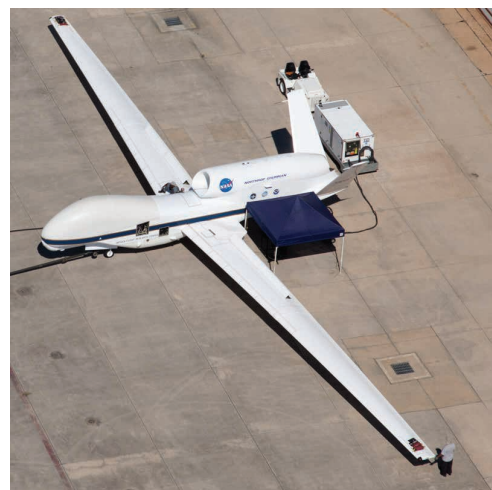
FIRST FLOWN IN 1998, THE U.S. AIR FORCE NORTHROP GRUMMAN RQ-4 GLOBAL HAWK IS STILL RELIED UPON AS A REMOTELY-CONTROLLED RECONNAISSANCE DRONE THAT IS SUITED FOR VERY HIGH ALTITUDE, LONG DURATION FLIGHTS. PILOTING THESE VEHICLES FROM THE GROUND HAS ALLEVIATED THE CONSTRAINTS OF HUMAN ENDURANCE WITHOUT THE RISK TO LIFE. GLOBAL HAWKS HAVE ALSO BEEN USED EXTENSIVELY BY NASA FOR HURRICANE AND SEVERE STORM STUDIES UNDER THE HS3 MISSION. IMAGE CREDITS: U.S. AIR FORCE/BOBBI ZAPKA/NASA GODDARD SPACEFLIGHT CENTER
