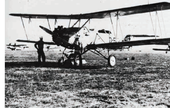
THIS EARLY PHOTOGRAPH TAKE CA. 1938 CAPTURES A U.S. NAVY CURTISS N2C-2 FLEDGLING THAT WAS CONVERTED TO RADIO-CONTROLLED TARGET DRONE. EARLY MILITARY DRONES WERE COMMONLY USED AS TARGET PRACTICE FOR HUMAN PILOTED AIRCRAFT. IMAGE CREDIT: U.S. NAVY
